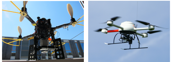
(a) AscTec Pelican drone with an FLIR Photon 640 thermal camera. (b) MD4-200 drone with an RGB camera.
