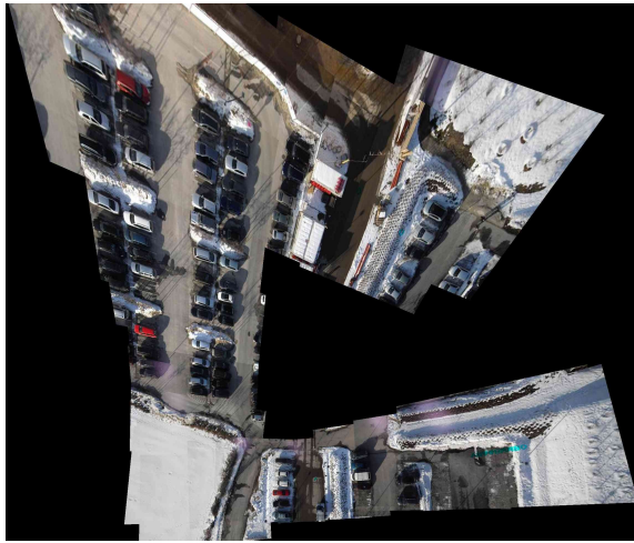
(a) Images are mosaicked with 2nd order radial distortion correction and without depth consideration.
