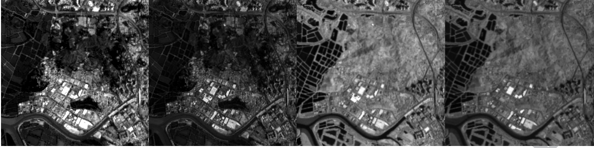
Fig. 11. Comparison of fusion results on Hyperion and SPOT5 data. From the top downwards, the rows illustrate the input Hyperion image, the fusion result of SUM, the fusion result of SRSR and the fusion result of DPLM, respectively; from left to right, the columns show the images of bands 8, 31, 56 and 120, respectively.
