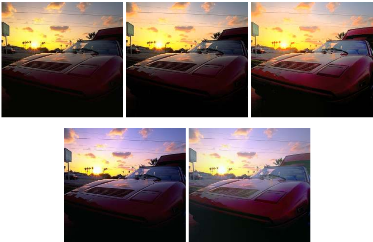
Figure 5: Comparison between the results obtained by processing independently each channel ( RGB ), and by processing the intensity component ( I ), with default parameters. Top left: original image. Top center: normalized image in I , top right: result of “Enhanced dark” in I . Bottom left: normalized image in RGB . Bottom right: result of “Enhanced dark” in RGB .
