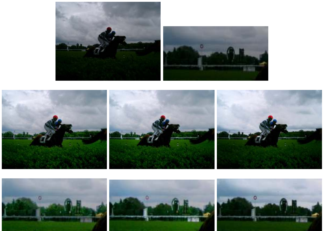
Figure 2: First row: original image and a detail of the image. Second row: selective contrast adjustment results with several T values ( a = 2.5 ). Left: T = 50 . Center: T = 100 . Right: T = 150 . Bottom: detail of the second row comparison.
