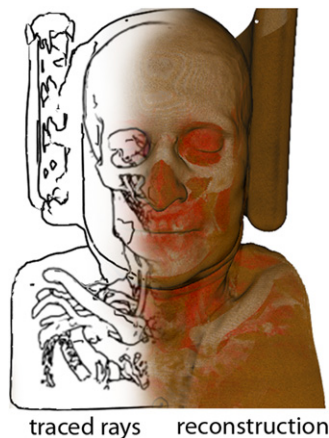
Fig. 1. This figure illustrates the basic idea of our method. Rays do not have to be equally distributed over the scene in ray-based rendering environments to get a visually pleasing result. It is sufficient to trace rays only in areas that have been proven to convey the shape of an object (left) for a good approximation of the result (right).
