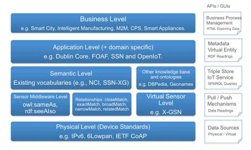
Figure 7 IoT Stack for Service Delivery Model and Interoperability
