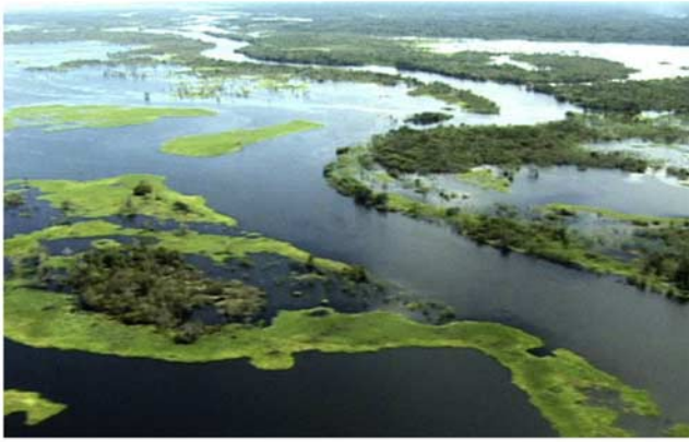
Figure 1. Inundated floodplain of the Amazon River. This geomorphology is highly complex, lacking well-defined channels; rather diffusive flow conditions are prevalent. Stream gauges are incapable of measuring these flow conditions and related storage changes. In fact, in situ gauges are not present anywhere on the Amazon floodplain. Photograph courtesy of L. Hess.
