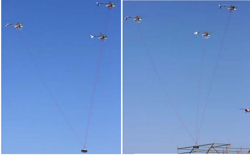
Fig. 3 Three autonomous helicopters from the Technical University of Berlin ( TUB-H model) transporting a wireless camera to the top floor of a building with a height of 12 meters in May 2009. A device on-board each helicopter is equipped with a force sensor to estimate the influence of the other helicopters and the load itself – term \gamma_i in eq. 4. The images show the mission during the actual load transportation (left) and shortly before the load deployment (right). A fourth helicopter which was used to acquire airborne video footage of the mission is visible on the right.
