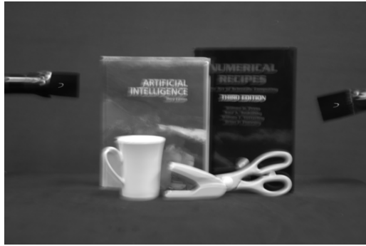
Fig. 11 Captured real image. Point light sources were placed on either side of the subject to estimate the PSF.
