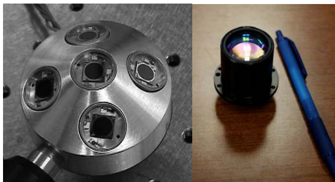
Figure 2: a) Corner cube MRR array b) Cat’s eye MRR.
