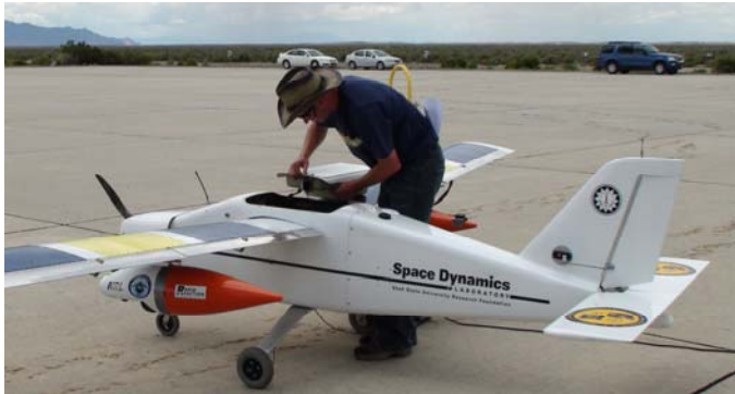
Figure 6. Dakota UAV with MRR lasercom wingpods
