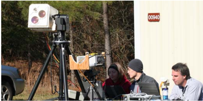
Figure 3. Dual mode optical interrogator (DMOI) on tripod
