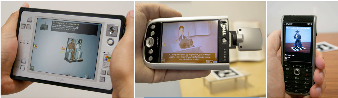
Figure 2: Evolution of Mobile AR Systems: Desktop Windows driven Tablet PC with weight about 1.2kg, ~1500 Dollar (left), PDA with external camera and limited communication capabilities (middle), Smartphone with built-in camera and various communication channels (GSM/3G and Wi-Fi) and low weight (100g), ~300 Dollar (right). (Image courtesy of Graz University of Technology)
