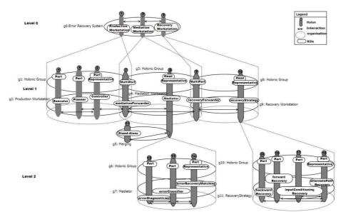
Fig. 1. Holarchy of Error Recovery System
