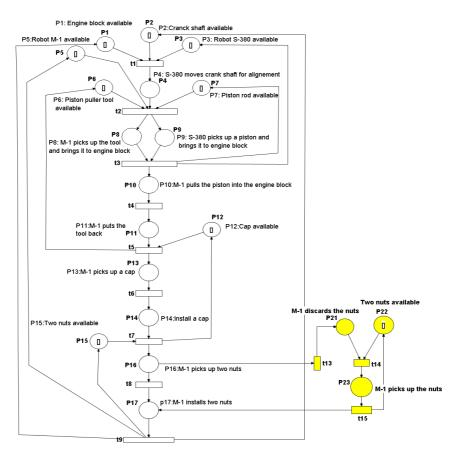
Fig. 4. Physical system model with error recovery module
