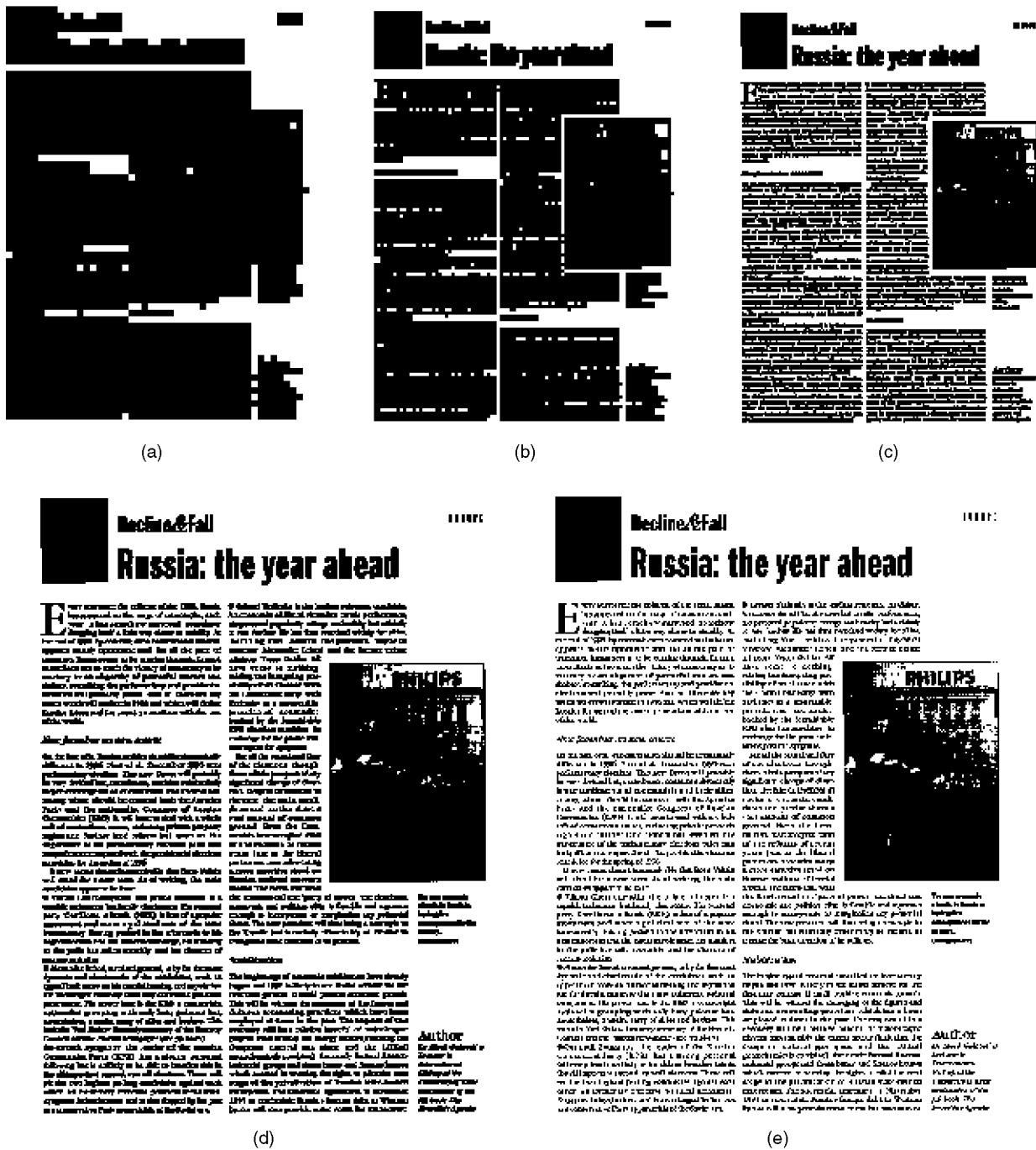
Fig. 3. Multiscale images: (a) top-level = level 4 (50x66), (b) level 3 (100x131), (c) level 2 (199x261), (d) level 1 (398x522), and (e) bottom-level = level 0 (796x1043).
