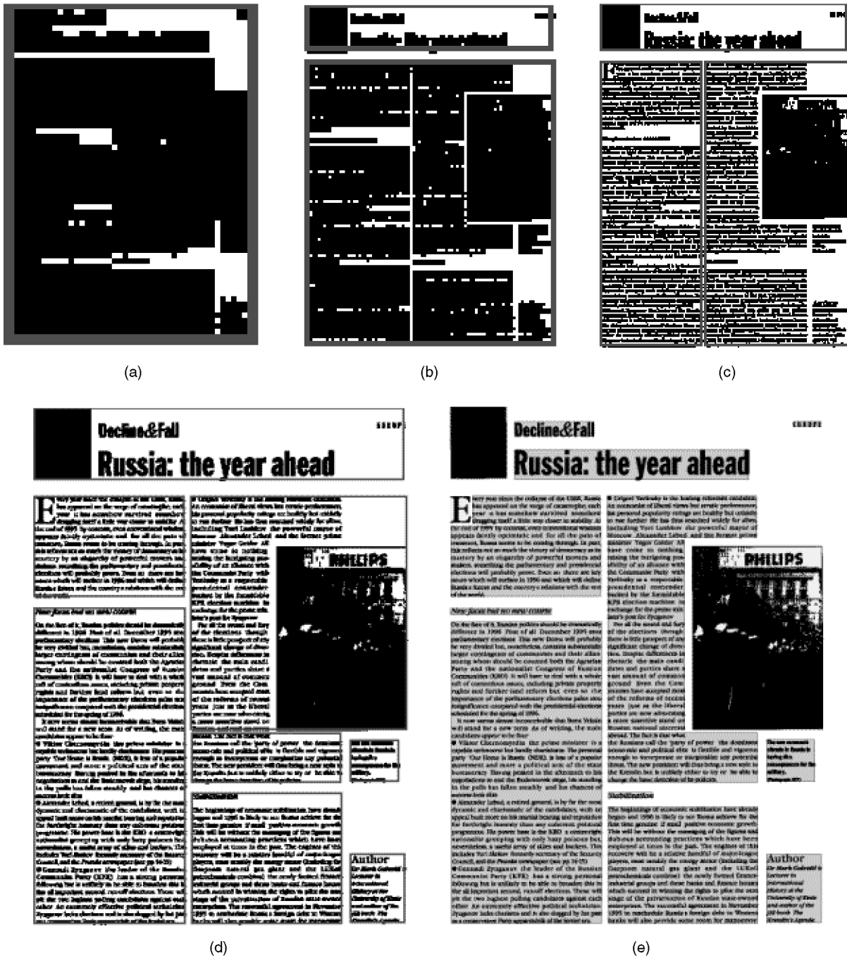
Fig. 15. An example to show the processes of the proposed method: (a) level 4 (50x66), (b) level 3 (100x131), (c) level 2 (199x261), (d) level 1 (398x522), and (e) level 0 (796x1,043).
