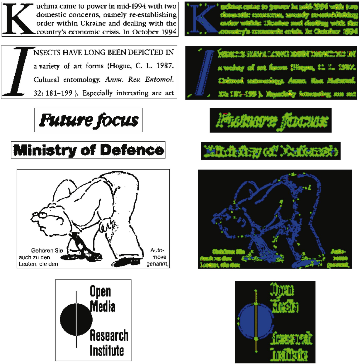
Fig. 13. Original images (left) and their classification results (right) (blue: image, green: text, red: horizontal ruling line, yellow: vertical ruling line, and black: background).
