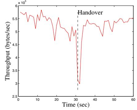
Fig. 7. Average throughput received in the MH in SEMO6.
