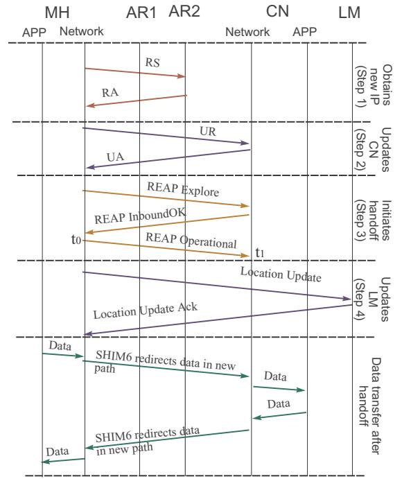
Fig. 1. Message flow of L3 handover of SEMO6.
