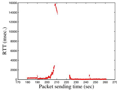
Fig. 10. RTT observed in CN in MIPv6.
