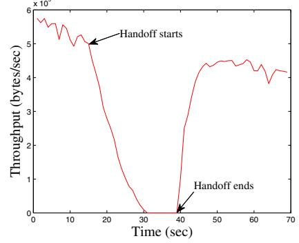
Fig. 8. Average throughput received in the MH in MIPv6.
