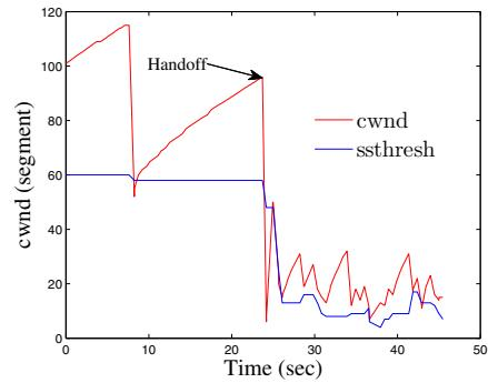
Fig. 11. cwnd and ssthresh in CN of SEMO6.
