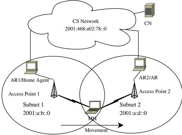
Fig. 2. SEMO6 Testbed architecture.
