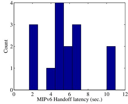
Fig. 6. Handoff latency histogram of MIPv6.
