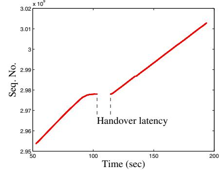
Fig. 4. Data received in MH with the TCP sequence number in MIPv6.
