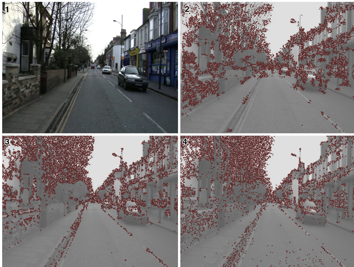
Fig. 3 From top to bottom: 1—test image of the detector benchmark. 2—Points extracted with an ideal detector based on the matching error map (10k points with the smallest matching error). 3—10k FAST keypoints. 4—10k MIEL keypoints
