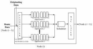
Figure 2. Queuing model for a particular node.
