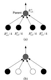
Figure 3. Any of the child nodes is termed as i, and the grey colored node is the parent of i, (a) All child nodes are active (black colored nodes) (b) Two child nodes are idle (white).
