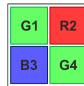
Figure 2. Bayer-pattern block CFA.
