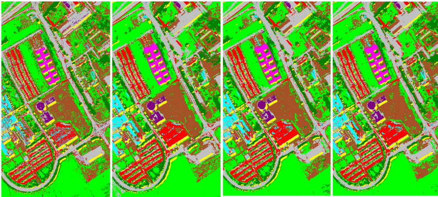
Fig. 11. Classification map of the standard SVM and the proposed classification method with 10-, 12-, and 14-level segmentation by FODPSO.
