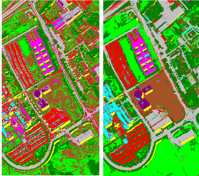
Figure 1.10: An example of classification maps, with (the right image) and without (the left image) considering spatial information. As can be seen, the classification map obtained by considering the both spectral and spatial information is much smoother than the classification map obtained by considering only spectral information. Considering the spatial information can reduce the labeling uncertainty that exists when only spectral information is taken into account, and helps to overcome the salt and pepper appearance of the classification map.
