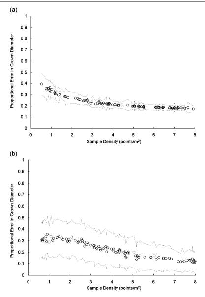
**Fig. 8** Graphs showing the bias in estimating crown diameters. Each point shows the mean error (per stand) in crown estimation for trees that have been correctly classified based on their x, y location. The outer lines show the standard deviation of error for estimated crown diameter for each stand. The graphs illustrate the relationship between crown error and point density for Basal Areas of **a** 10 and **b** 20 m<sup>2</sup>/ha
