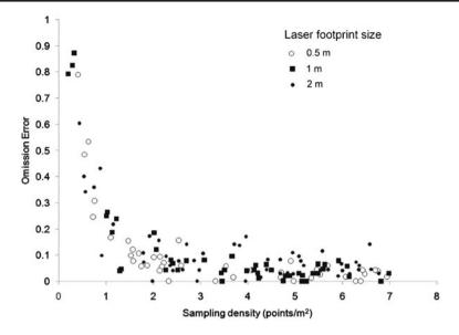
**Fig. 5** Effect of LiDAR footprint size on tree identification. The graph shows the success of the tree identification algorithm over a range of sampling densities and assuming footprint sizes of 0.5 m (*open circles*), 1 m (*closed squares*) and 2 m (*closed circles*). The graph suggests that footprint size has a minimal effect on the success of tree detection
