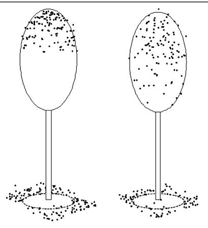
**Fig. 1** Diagram showing simple geometric trees and the distribution of synthetic LiDAR data sampled from the trees. The tree on the left shows LiDAR samples with x,y error and backscatter error only. The tree on the right shows LiDAR samples with additional penetration error
