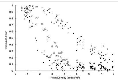
**Fig. 9** Graph showing how changes to the definition of success criteria influence omission errors. Omission error (whether a tree is successfully identified) is defined by an acceptable level of accuracy between estimated vs actual tree characteristics. The graph shows acceptance criteria of 20 (*triangles*), 25 (*open circles*) and 30 (*closed circles*) percent
