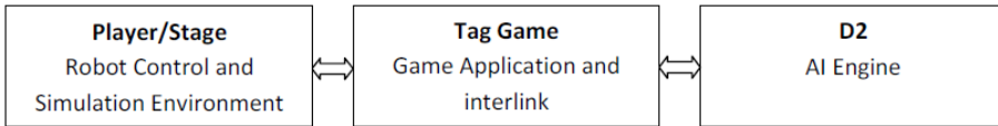
Figure I.2: Illustration of the three components of the framework; a robot controller (Player/Stage), an interlinking game application (Tag Game) and an AI engine (D2)
