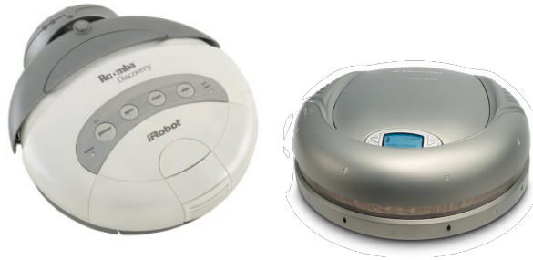
Figure L.4: Robot vacuum cleaners. From left: Roomba from iRobot [13] and Trilobite from Electrolux [14]
