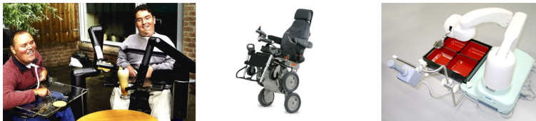
Figure L.2: The iARM from Exact Dynamics [3], the iBOT wheelchair [4] and the mySpoon robot [5]
