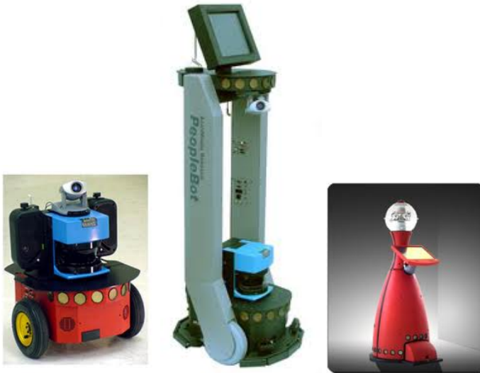
Figure 3.7: Three commercial general purpose mobile platform robots. From left to right: Pioneer P3-DX and PeopleBot by Adept Mobilerobots [5] and Scitos G5 by Metralabs [184]
