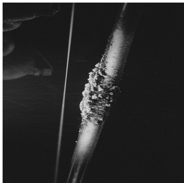
Fig. 21. Photograph of deposit forming from wheat straw on a simulated boiler tube [81].
