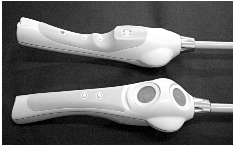
Figure 2. Example of a biosonar-inspired mobility aid for the blind, the ‘Ultracane’ [27]; the handle includes two ultrasonic transducers—one forward-looking, one upward-looking—and a tactile display consisting of four transducers. Photograph by Dean Waters, reproduced with permission by the copyright owner.
