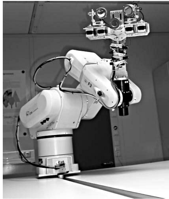
Figure 4. Biosonar head mounted on a 6-degree-of-freedom industrial robot arm and a linear track for expansion of work envelope [52].
