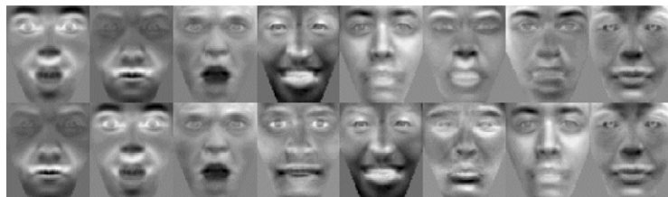
Fig. 4. From top to bottom, the first eight eigenfaces and the first eight optimal ones (after the sorting process). The learning set contains N = 210 facial masks: N_c = 35 per facial expression for six expressions.
