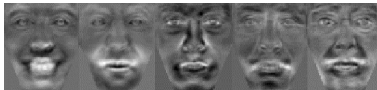
Fig. 5. Illustration of the five Fisherfaces, corresponding to five axes of the subspace generated by Sorted PCA plus LDA method, which are used as basis of the final discriminant subspace. The learning set contains N = 210 facial masks: N_c = 35 per facial expression for six expressions.
