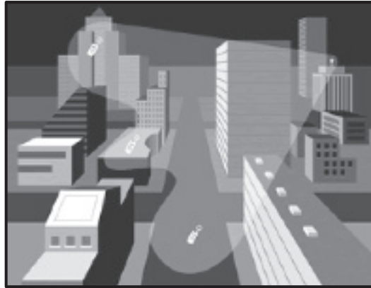
FIGURE 9.3: The use of standard or custom patterns to fit the topology of sector coverage [228].
