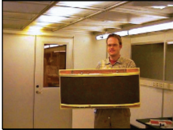
FIGURE 4.22: Picture of an eight-element array antenna at 1.8 GHz. (Antenna property of Telia Research AB, Sweden) [80].
