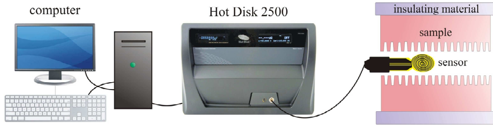
Fig. 3. The schematic of the experimental setup using a Hot-Disk 2500 thermal-constant analyzer based on a transient plane source method.
