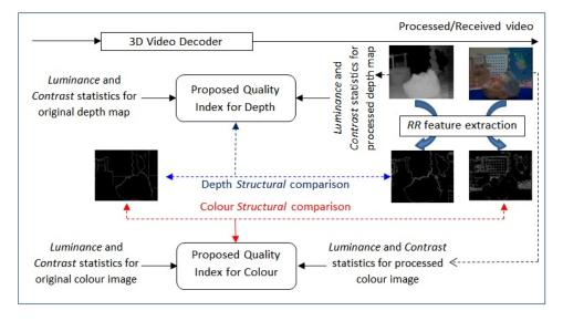
Fig. 3. Reduced reference edge based 3D video quality metric [12].
