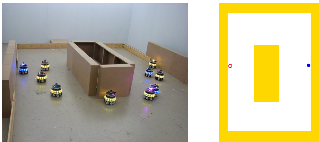
Fig. 23. Arena used in the real robot experiments with obstacle: photograph (left) and as reproduced in simulation (right). The circle and the disk symbols in the right image indicate the position of the food and the nest robots.
