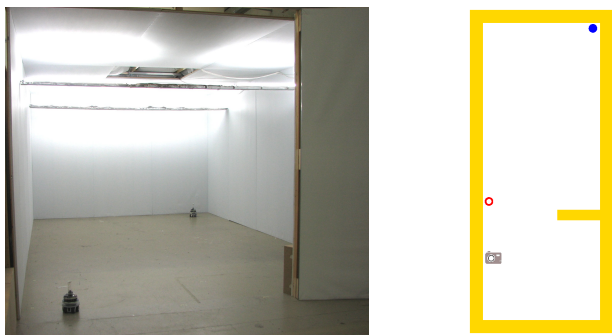
Fig. 21. Arena used in the real robot experiments: photograph (left) and as reproduced in simulation (right). The photograph was taken from the position of the camera icon in the right image. In this image, the circle and the disk symbols indicate respectively the position of food and nest robots.
