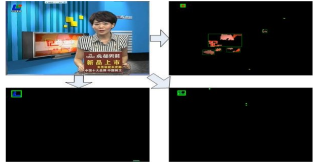
Fig.4. Divide the test image into three sub-images by the color features of candidate logo
