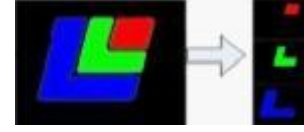
Fig. 3. Example of extracting color features by selecting the first three dominant colors with the largest proportion.
