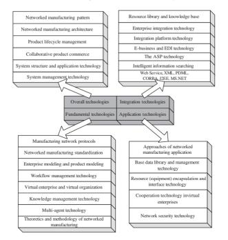
Figure 3. Technologies of networked manufacturing.
