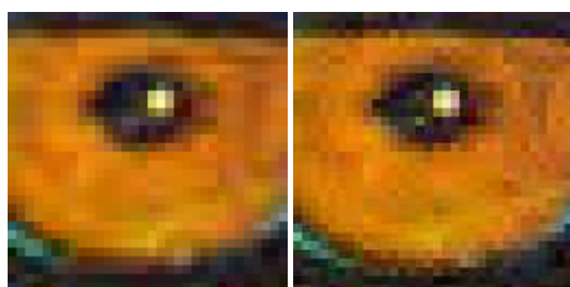
Fig. 8. The comparison between JPEG quantization table with QF = 50 (left) and TMT psychovisual threshold with QS = 0 (right) zoomed in to 400%
