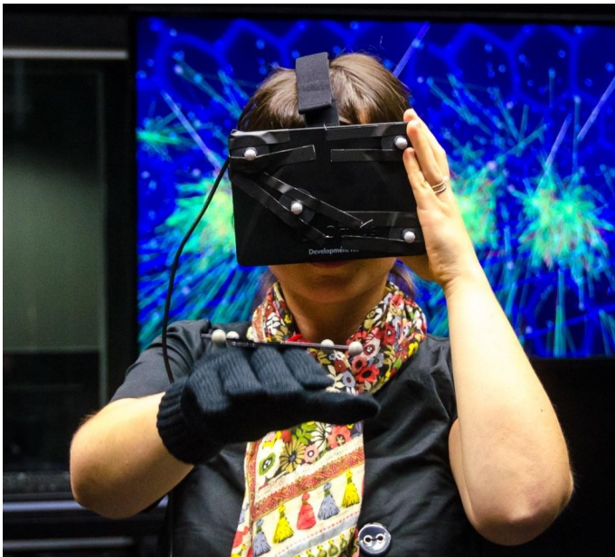
Figure 7: A user navigating through the virtual representation of the NeuCube network, using an intuitive, hand position based 3D cursor.
