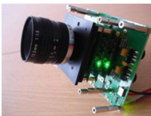
Fig. 1 Close-up of the wireless camera with an FPGA board from Delta Technologies [1]
