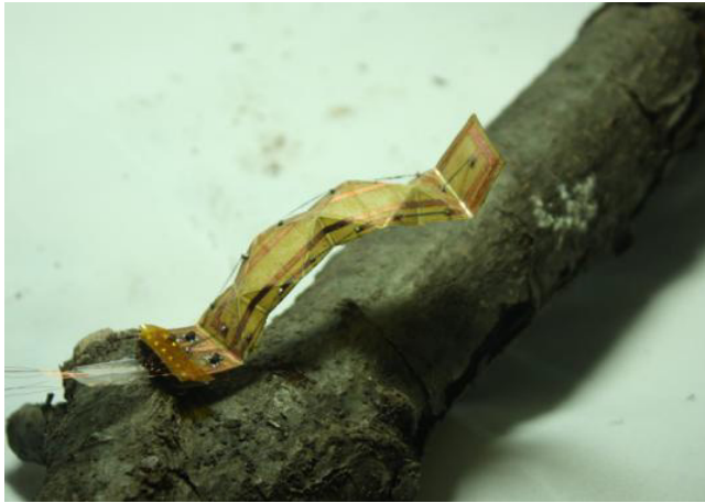
Figure 8. Omegabot, a biomimetic inchworm robot, grasps the branch of a wood, raises its head, and turns right. Bottom right: Proleg of Omegabot [38].
