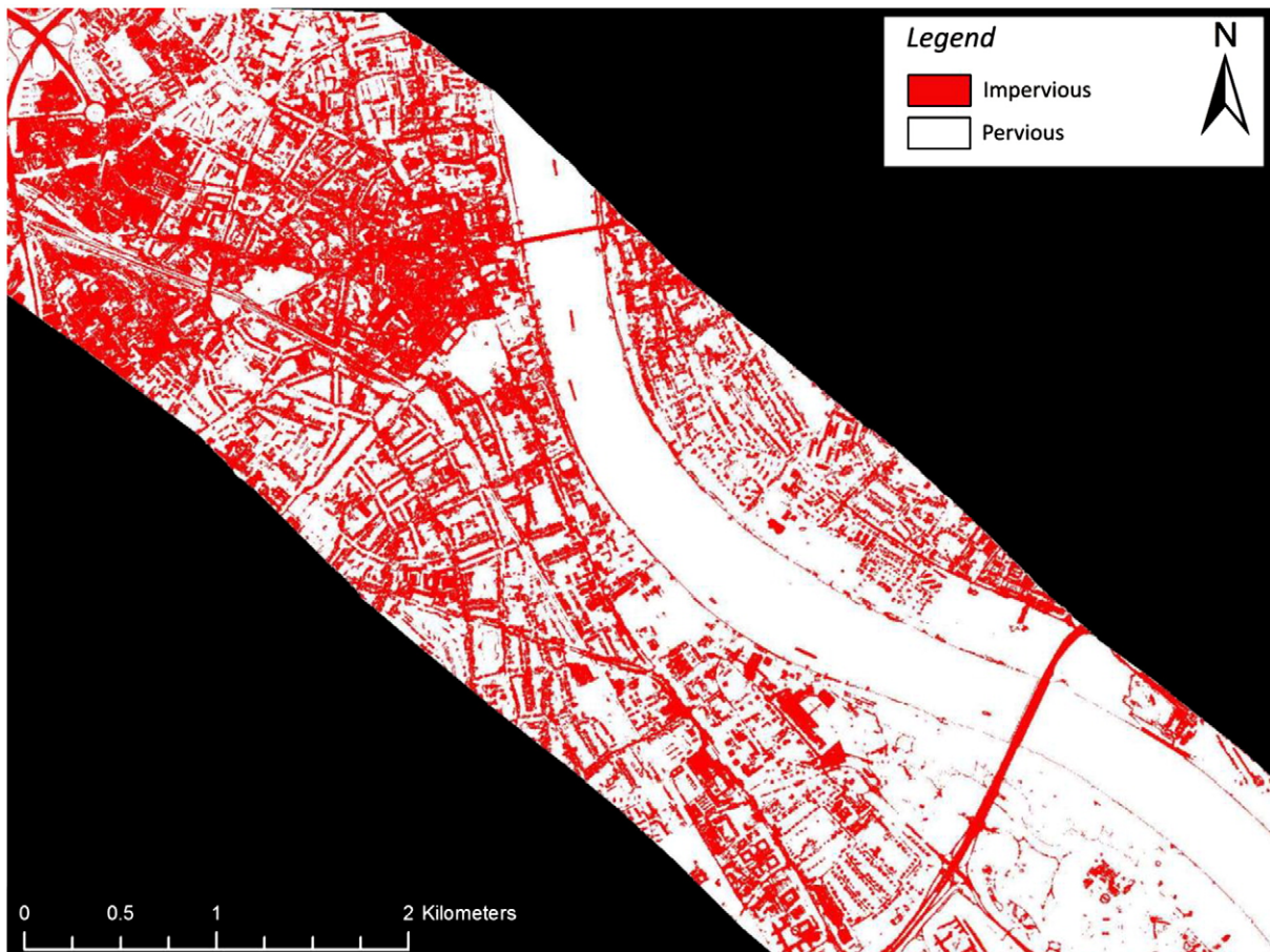
Fig. 4. Merged classification result of level 1 as derived from two- and three-endmember model MESMA, showing impervious and pervious surfaces in the area of Bonn with an overall classification accuracy of 97.2%.
