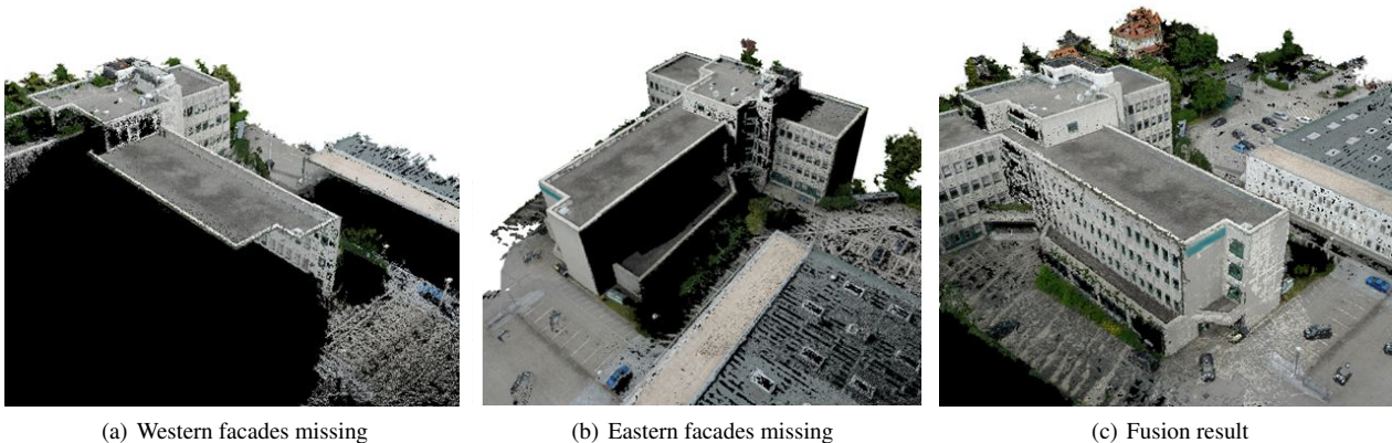
Figure 1: Typical results for the automatic fusion of two partial reconstructions, based on MAV imagery. Best viewed in color.
