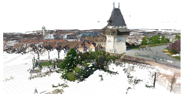
Figure 5: Fusion and geo-referencing of partial reconstructions. The medieval clocktower in front has been fused and aligned to the geo-referenced, approximated DSM of the city in the background.
