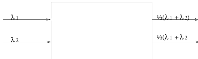
Figure 3.1: A 2 \times 2 3-dB coupler
