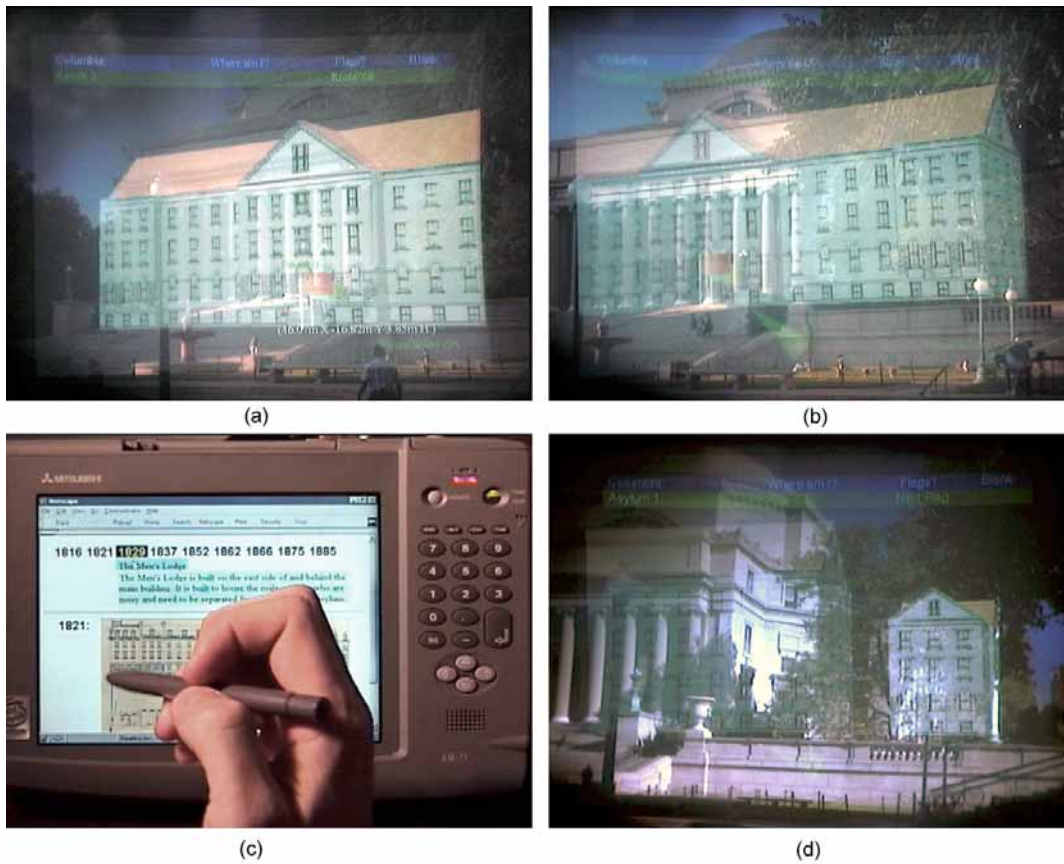
Figure 5.5: (a)–(b) A 3D model of the main Bloomingdale asylum building overlaid on Columbia’s campus by the see-through head-worn display. (c) An interactive timeline displayed on the hand-held computer when user selects the year the Men’s Lodge was built. (d) The AR scene responds by displaying the Men’s Lodge and fading out the main asylum building.
