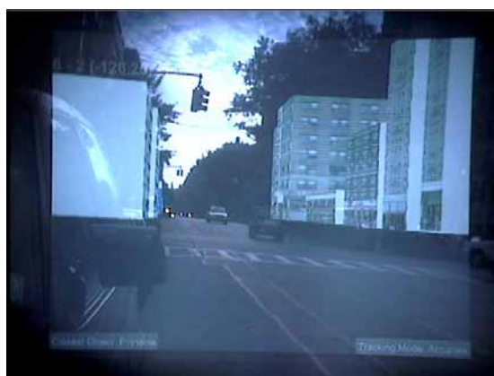
Figure 5.18: Simple building models overlaid on view of Broadway during registration tests for the restaurant tour guide.
