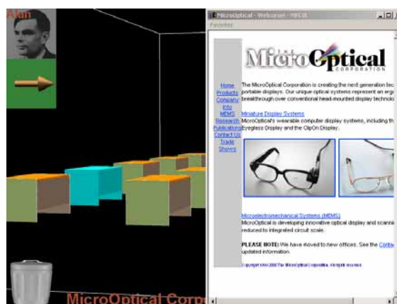
Figure 5.14: Screenshot (non-overlay) of JABAR interface shown at ISWC 2000. The graphics were overlaid on top of a trade show environment. The view shown was for giving a “through-walls” overview of the trade show from outside the hall. We display virtual desks for each booth. On the right-hand side of the screen is an integrated web browser showing information about the currently selected exhibitor.
