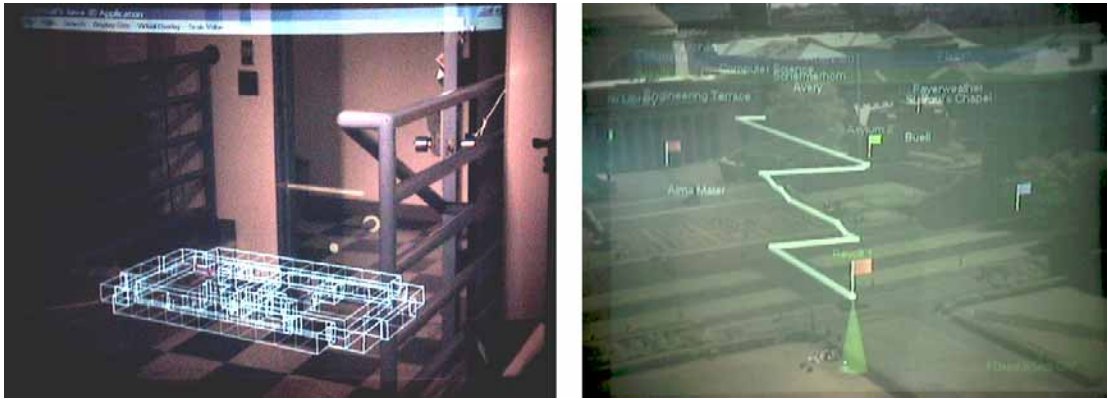
Figure 2.2: Navigational AR interfaces, imaged through head-worn displays. (a) Indoor guidance using overview visualization and arrows. (b) Virtual trails and flags outdoors (viewed from the roof of a building).
