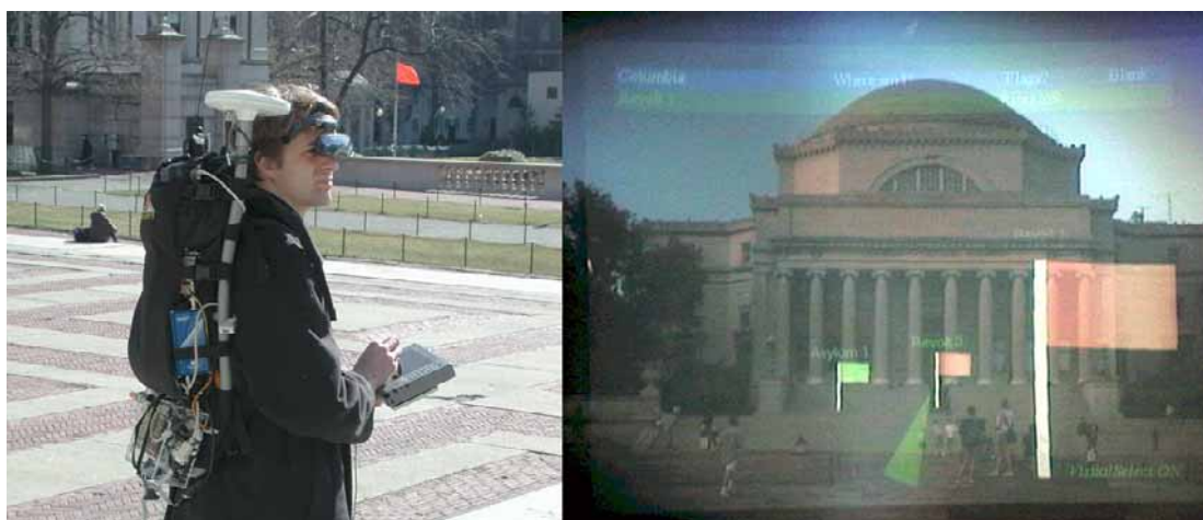
Figure 1.1: (a) The author with MARS backpack, tracked head-worn display, and hand-held computer, watching (b) an augmented campus scene (from the Situated Documentaries II application)
