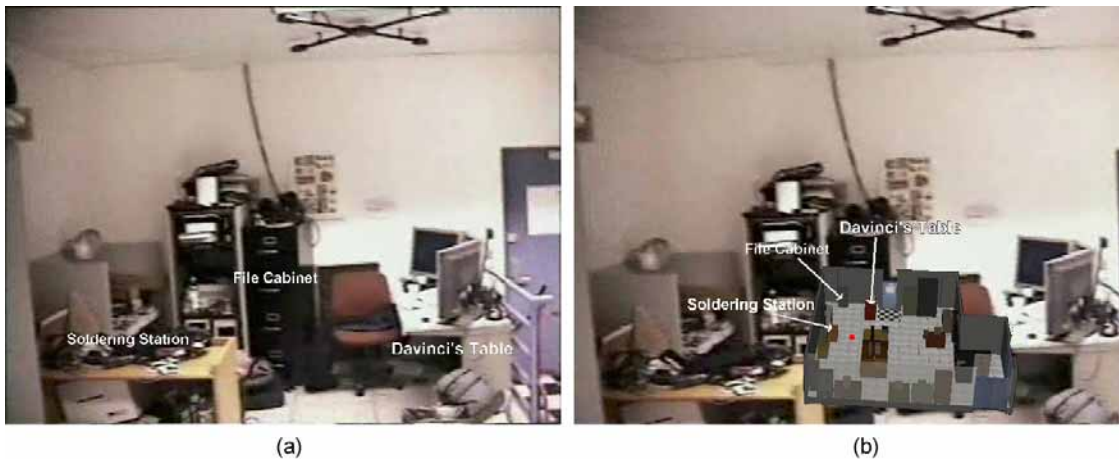
Figure 6.10: User interface adapting to different tracking accuracies. (a) Tracked by accurate 6DOF ceiling tracker: World-stabilized annotations. (b) Tracked by coarse wide-area infrared tracker: Screen-stabilized WiM.
