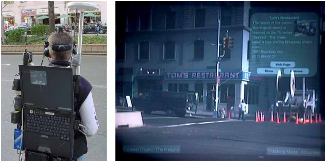
Figure 2.3: Mobile AR restaurant guide. (a) User with MARS backpack, looking at a restaurant. (b) Annotated view of restaurant, imaged through the head-worn display.
