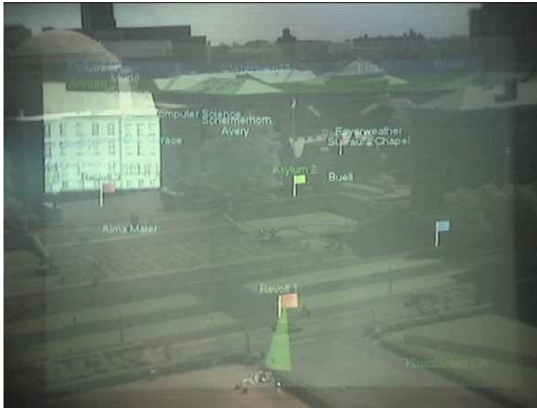
Figure 5.20: AR view from an unusual vantage point (roof of a campus building), exemplifying some of the problems of general mobile AR UIs, such as limited field of view, visual clutter, information overload, unwanted obstruction, and misplaced labels.
