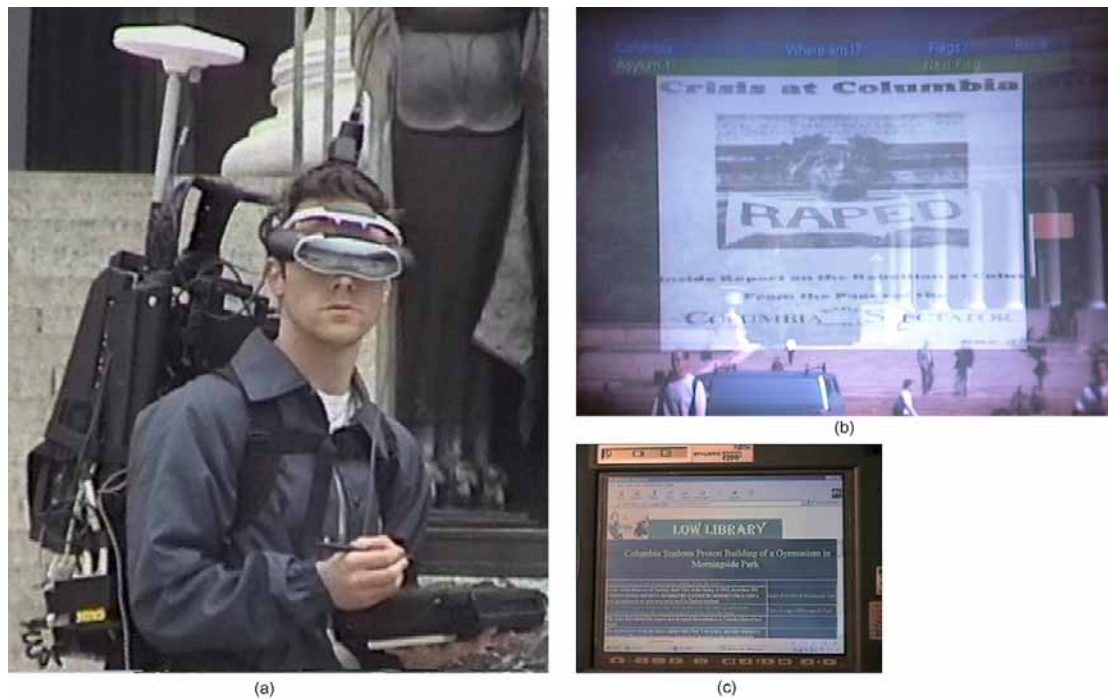
Figure 2.4: Situated Documentaries I. (a) User with backpack MARS. (b) View through head-worn display, showing multimedia story about Columbia 1968 student revolt. (c) Additional information on complementary hand-held display.
