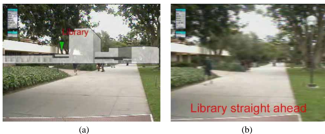
Figure 6.9: User interface adapting to user’s head motion. (a) Standing still: world-stabilized overlays of building model and target pointer. (b) With considerable head motion the view changes to a completely screen-stabilized message.
