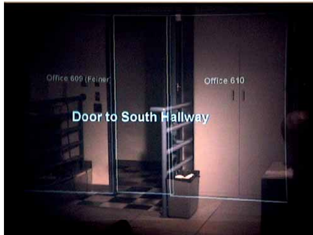
Figure 5.15: Augmented reality user interface in accurate tracking mode (imaged through see-through head-worn display). Labels and features (a wireframe lab model) are registered with the physical environment.
