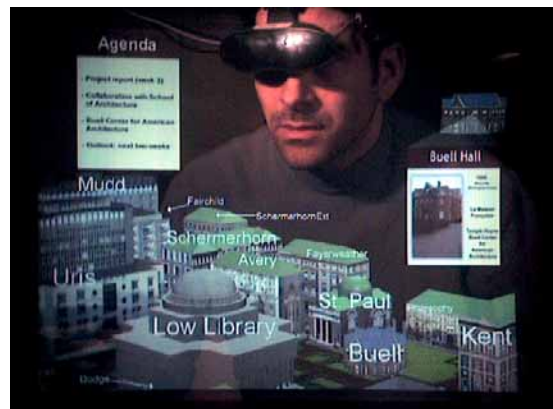
Figure 5.25: View management in a collaborative system (imaged through see-through head-worn display). Labels are laid out dynamically to annotate the buildings of a campus model as seen by the observer. UI elements avoid overlapping the colleague's head and the campus model.
