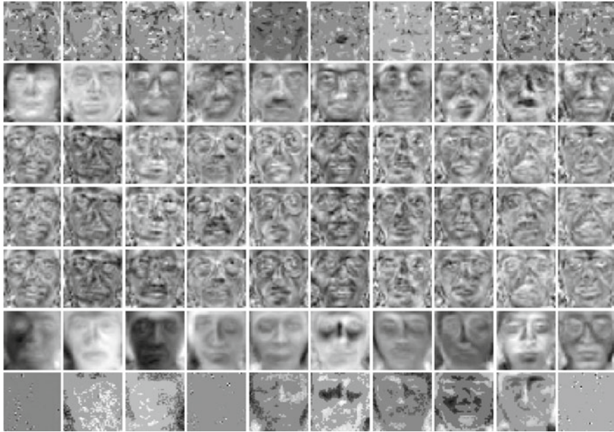
Fig. 10 Plots of first 10 bases obtained from 7 dimensionality reduction algorithms on YALE For each column, from top to bottom: MEN, DLA, LPP, NPE, FLDA, PCA, and SPCA
