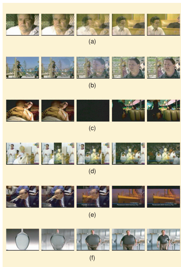
[FIG2] Examples of gradual transitions from the TRECVID 2003 corpus: (a) a dissolve between shots with similar color content; (b) a dissolve between shots with dissimilar color content; (c) fade; (d) a wipe of the “door” variety; (e) a wipe of the “grill” variety; and (f) a computer-generated special effect transition between shots.
