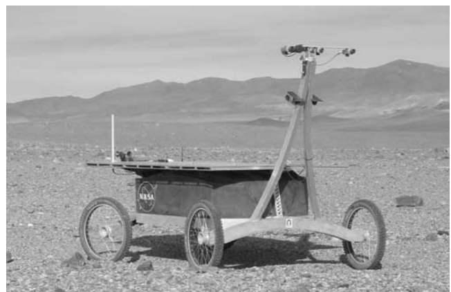
Figure 2. Zoë rover in the Atacama Desert. The rover and its instrument payload were designed together to be able to conduct multikilometer survey traverses in desert environments. Sensor mast is at typical eye-level and optics match human foveal resolution. Wide-tread pneumatic tires, not suitable for Mars, are ideal for terrestrial deserts.
