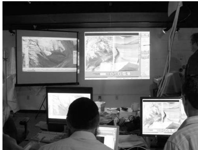
Figure 9. Remote operation center in Pittsburgh. Computers projected data directly on the wall screens to facilitate the team's discussions during data analysis, meetings, and daily traverse planning. The desktops were also used for download of rover data at the end of the day and upload of the daily traverse plans. Laptops were used by science team members to complete personal data analysis and reports.
