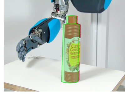
Fig. 7. Graphical representation of the initial object pose by the vision system
