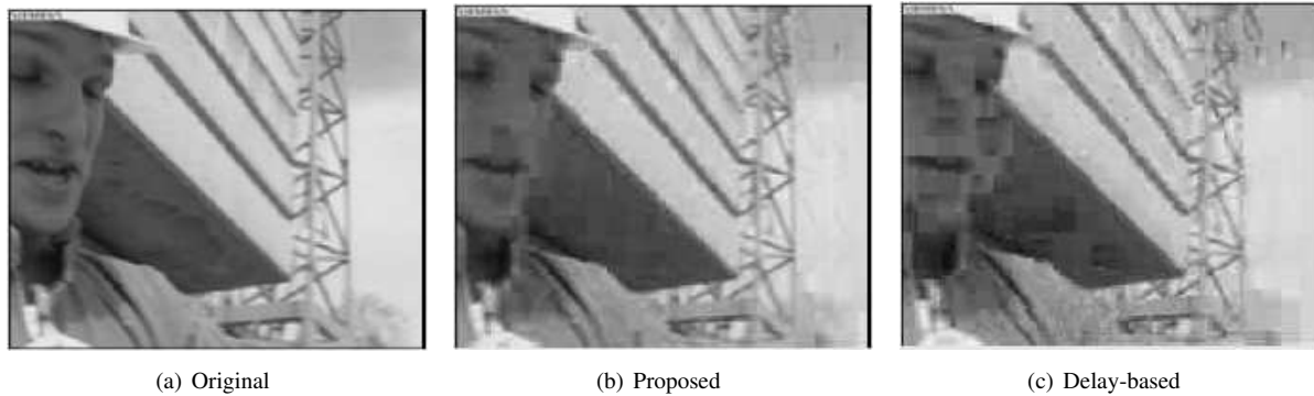
Figure 9. Frame 92 in the “Foreman” sequence: a) original frame; b) expected frame at the decoder using the JSCPA approach; c) expected frame at the decoder using the ISCPA approach.
