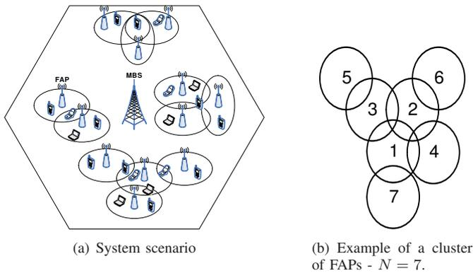
Fig. 1. Femtocell network.
