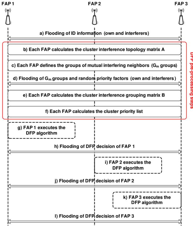
Fig. 2. Basic processing and communication protocol of the frequency planning technique in a distributed architecture.
