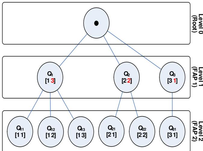
Fig. 3. Example of a dynamic search tree of the BnB-based DFP algorithm considering two interfering FAPs and four sub-carriers.
