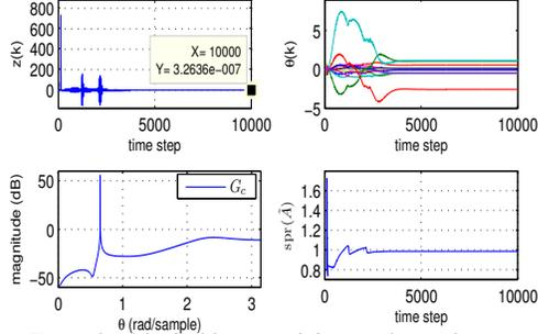
Fig. 11. Example 5.2: Stable, nonminimum-phase plant, command following with  $w(k) = \sin(0.65k)$ ,  $\eta_0 = 0.055$ . The performance  $z(k)$  converges to zero with this level of regularization even in the presence of large phase mismatch  $\Delta(0.65) = 152$  deg at the command frequency. However, the large phase mismatch results in longer adaptation period.
