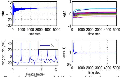
Fig. 15. Example 5.4: Command following and disturbance rejection with a 6-tone exogenous signal. In this case,  $\Delta_3(\theta) < 90$  deg for all  $0 \leq \theta \leq \pi$ , and the performance  $z(k)$  converges to zero.
