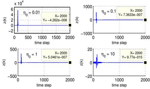
Fig. 10. Example 5.2: Stable, nonminimum-phase plant, command following with  $w(k) = \sin(2k)$ . Each subplot corresponds to a run with different  $\eta_0$ . The performance  $z(k)$  converges to zero in each case, and the transient performance is improved as  $\eta_0$  increases.
