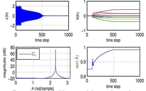
Fig. 12. Example 5.3: Stable, nonminimum-phase plant, unmatched disturbance rejection with  $w(k) = \sin(2.31k)$ . In this case,  $\tilde{H} = H_1$ , so that  $\Delta(2.31) = 13$  deg. The performance  $z(k)$  converges to zero.
