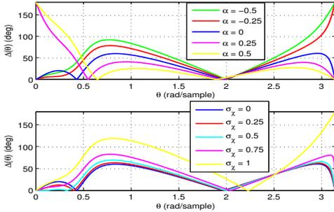
Fig. 16. This figure shows the effect of uniform additive error and random additive error in the Markov parameters for the plant in Example 5.4, and  $r = 3$ . For positive  $\alpha$ , degradation is highest at  $\theta = 0$ , whereas, for negative  $\alpha$ , degradation is highest at  $\theta = \pi$ . Degradation is low at the intermediate frequencies for all  $\alpha$ . With  $\sigma_\chi = 1$ ,  $\Delta(\pi) = 180$  deg, and degradation is lower at all other angles.
