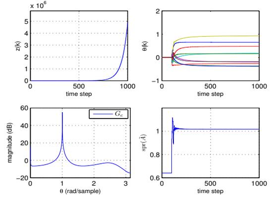
Fig. 3. Command following with  $w(k) = \sin(k)$ . In this case,  $\tilde{\mathcal{H}}$  is constructed such that  $\Delta(1) = 91$  deg, without using Markov parameters. The performance grows unbounded, and RCAC converges to a destabilizing internal model controller.
