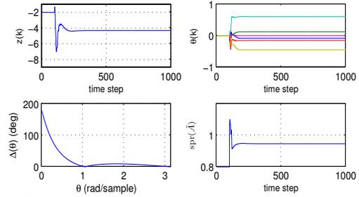
Fig. 7. Example 5.1: Stable, nonminimum-phase plant, step-command following. In this case,  $\tilde{\mathcal{H}} = H_1$ , so that  $\Delta(0) = 180$  deg. The performance is driven in the wrong direction due to 180-deg phase mismatch at DC.
