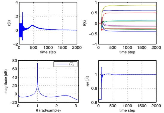
Fig. 4. Command following with  $w(k) = \sin(k)$ . In this case,  $\tilde{\mathcal{H}}$  is constructed such that  $\Delta(1) = 91$  deg, without using Markov parameters. In this case, adaptive regularization prevents RCAC from destabilizing the closed-loop system, and the performance  $z(k)$  converges to zero.
