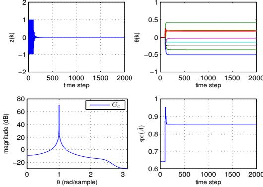
Fig. 2. Command following with  $w(k) = \sin(k)$ . In this case,  $\tilde{\mathcal{H}}$  is constructed such that  $\Delta(1) = 0$  deg, without using Markov parameters. The performance  $z(k)$  converges to zero, and RCAC converges to an internal model controller with high gain at  $\theta = 1$  rad/sample.
