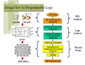
Fig. 8: Design Flow for Programmable Logic
