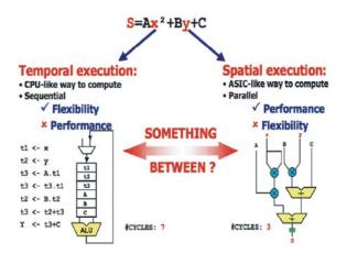
Fig. 1: ASIC vs. GPP Computing
