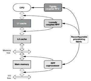
Fig. 6: Coupling Approach for Reconfigurable Fabric
