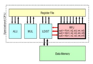
Fig. 5: Reconfigurable Processors Core
