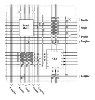
Fig. 4: FPGA Routing Structure
