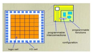
Fig. 3: FPGA Internal Architecture
