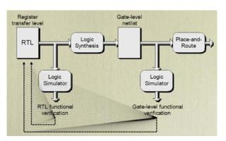
Fig. 7: RTL Based Design Simulations
