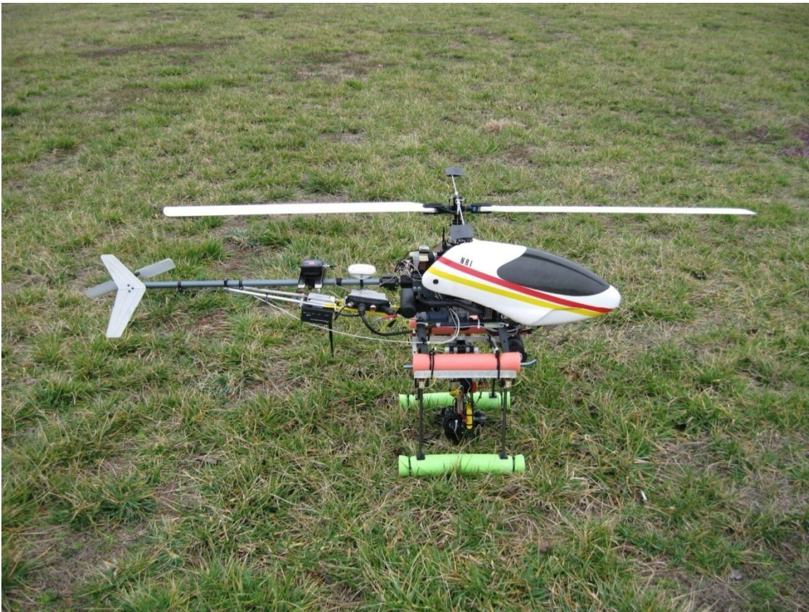
Fig. 3. The Aerial Surveillance Vehicle used for the demo project. A Vario Benzine trainer equipped with Global Positioning System, Altitude and Heading Reference System, Global Positioning System, modem, and Camera Gimbal.
