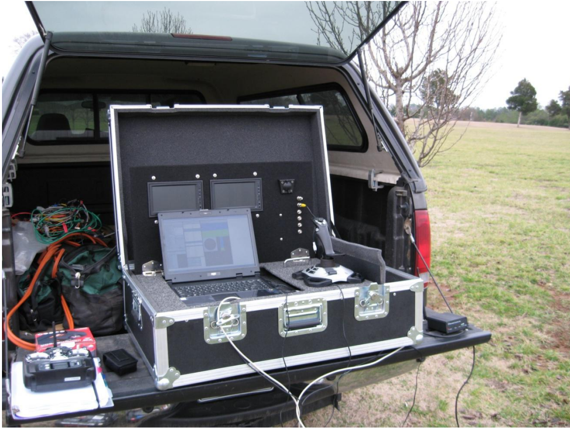
Fig. 4. The ground control station for semi-autonomous and full-autonomous flight control of the aerial surveillance vehicle. The laptop communicates joystick inputs to the Aerial Surveillance Vehicle through a modem. Live video from the Aerial Surveillance Vehicle is transmitted to the ground control station monitor for viewing.
