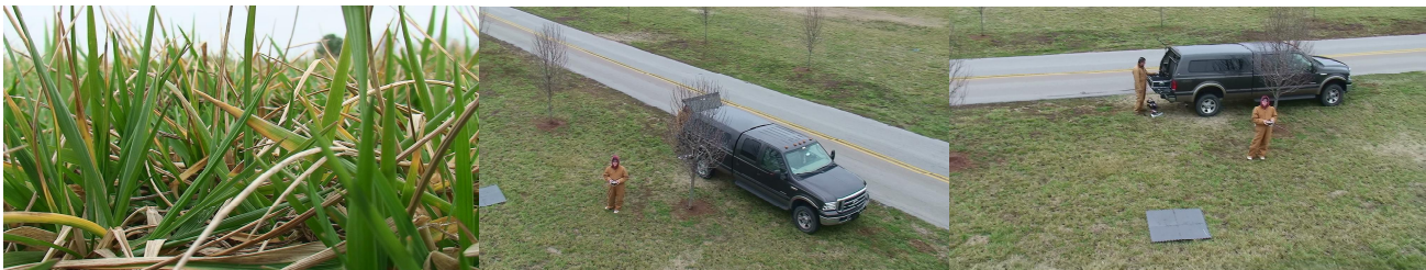
Fig. 6. Images from the video camcorder mounted on the gimbal below the aerial surveillance vehicle in semi-autonomous flight mode. The left image is while the ASV is idling on the ground. The center image is at 40 feet (12.2 meters) and 45 degrees of down camera angle. The right image is at 30 feet (9.1 meters) and 15 degrees of down camera angle. The images are still images from the recorded video file.
