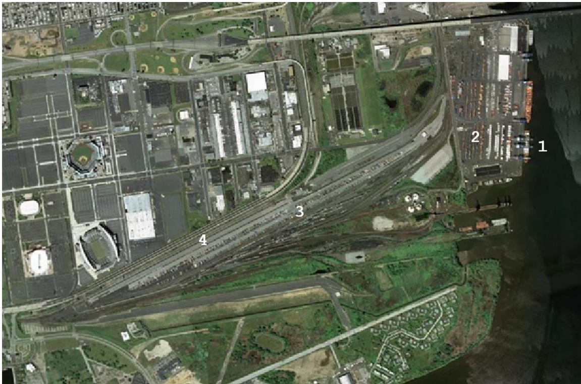
Fig. 1. Port of Philadelphia and adjoining CSX rail yard. Location 1 is the dock area for ship loading and unloading, location 2 is the container staging area where containers are stored awaiting pick-up, location 3 is the CSX container storage area where containers are picked-up or dropped-off as needed by rail operations, and location 4 is the CSX rail line used for loading the train cars and building trains for departure [source of aerial photo – Google Earth].
