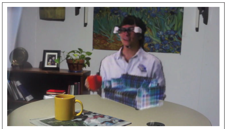
Figure 7. View through an experimental augmented reality head-mounted display showing a distant participant across the local table and a virtual couch model on the table.
