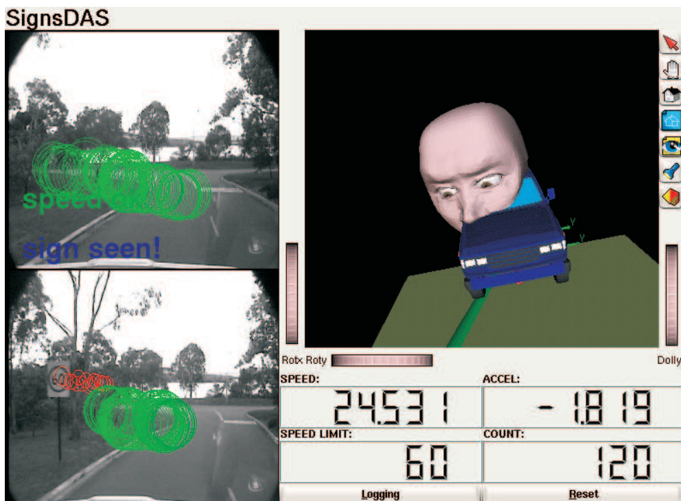
Fig. 20. Screen-shot showing “60” sign detected and seen by driver. Top left: Live video showing eye gaze (large circles) and status (overlaid text). Bottom left: Last detected sign (small circles) and eye gaze (large circles). Top right: 3D model of current vehicle position, eye gaze (oversize head) and sign location. Bottom right: Current detected speed limit, vehicle speed, acceleration and count down for speeding grace period in frames.
