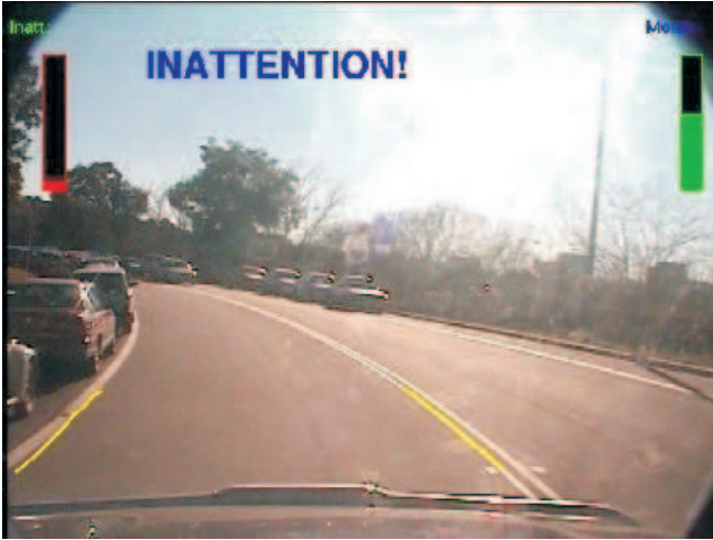
Fig. 31. Screen-shots of the Automated Co-driver. Prolonged inattention detected. Large circles: no circles are shown in this case as the driver's gaze is outside the field of view of the camera (consistent with the driver inattention detected).
