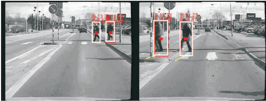
Fig. 11. Online pedestrian detection. The basis for the system used in the Automated Co-driver.
