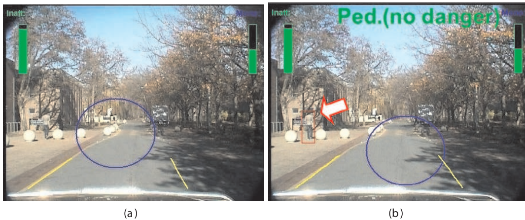
Fig. 35. Automated Co-driver screen-shot sequence. Circles represent driver gaze. (a) Approaching pedestrian detected. (b) Pedestrian determined to be no threat. Arrow added manually afterwards.
