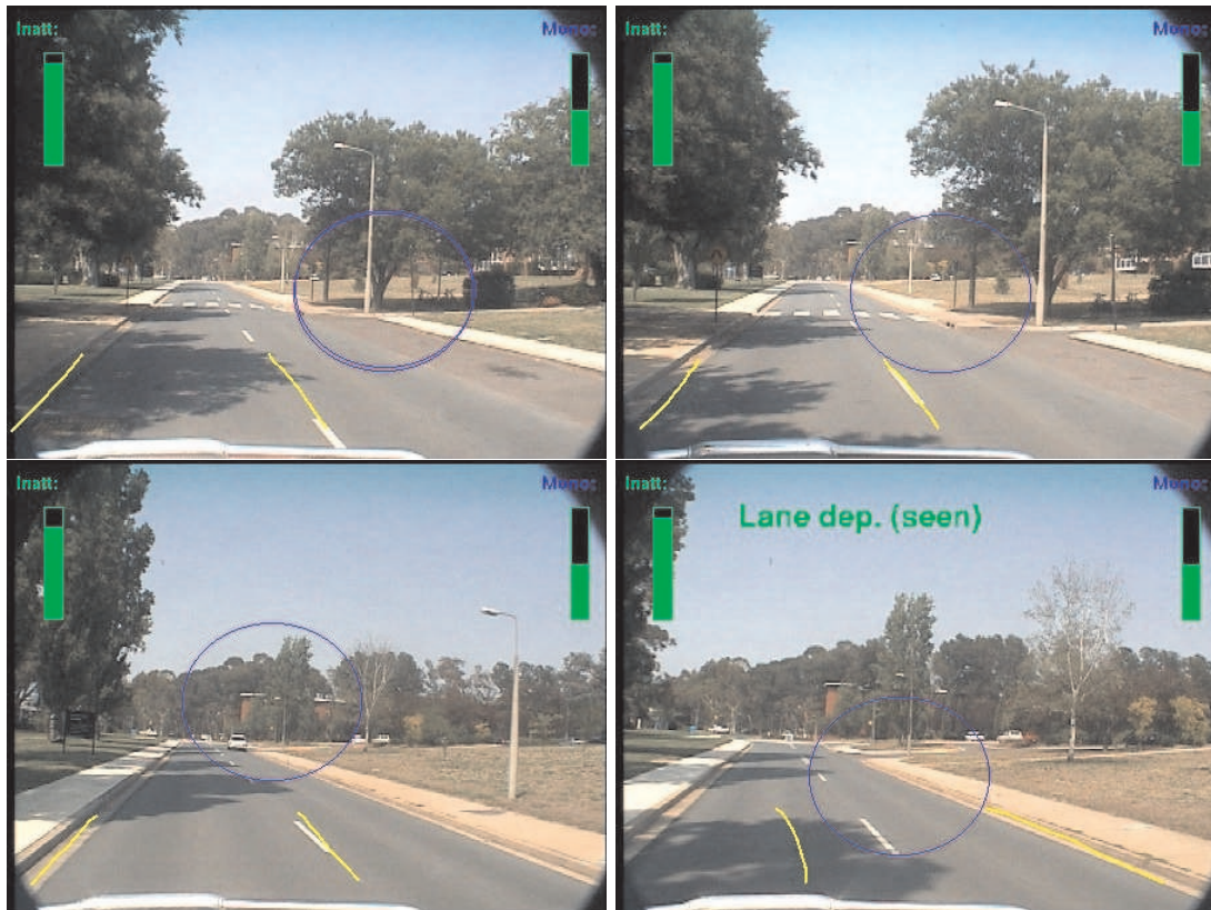
Fig. 33. A sequence of screen-shots of the Automated Co-driver. A lane departure that was seen by the driver is shown. Large circles: driver gaze.
