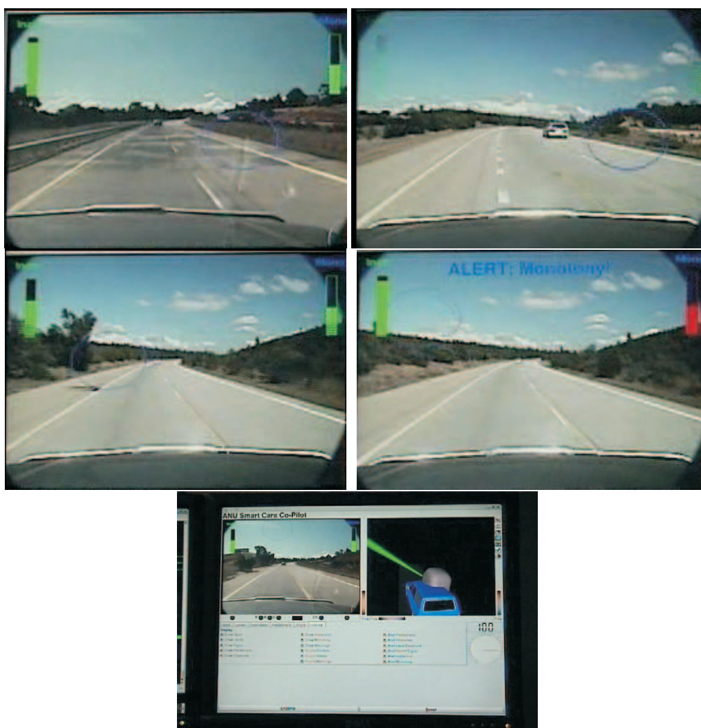
Fig. 37. Sequence of screen-shots of the Automated Co-driver showing a monotony warning occurring. Large circles: driver gaze.
