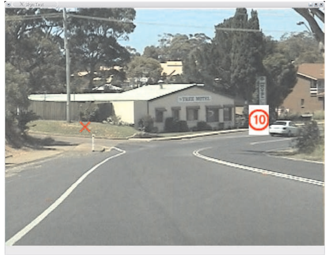
Fig. 14. Screen-shot of PC test application to gather data on gaze object recognition field of view. A test subject is requested to fix their gaze on the cross. The Speed sign periodically varies in position and speed (10,20,30,....,90). A road video sequence was played in the background to add context for the trials. The subject entered the “guessed” sign via a numeric keypad (“1”–“9”).
