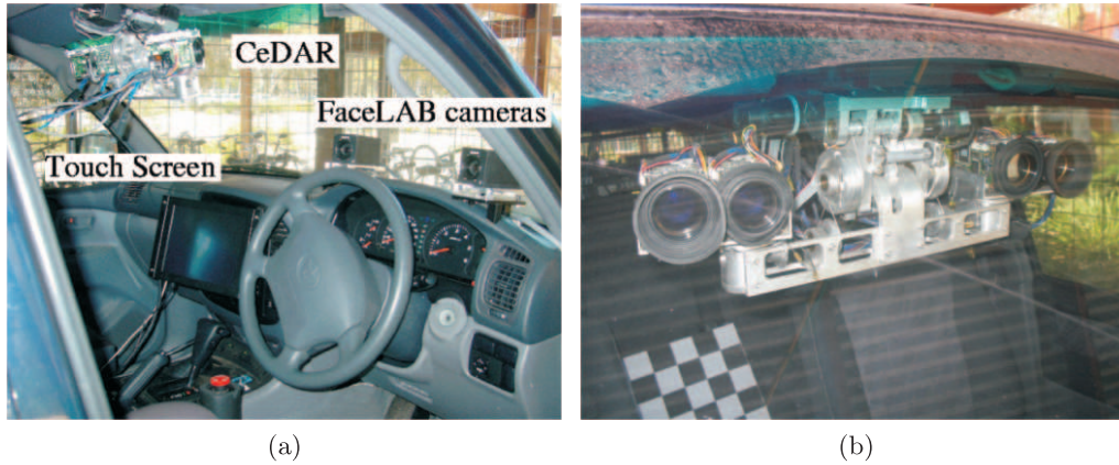
Fig. 6. (a) The cameras on-board the vehicle. The CeDAR active vision platform containing the stereo road scene cameras and faceLAB™ passive stereo cameras observing the driver. (b) CeDAR: Cable Drive Active vision Robot in vehicle. Four cameras are arranged in two stereo pairs. Cameras are fitted with polarizing filters and far-field cameras use glare hoods.
