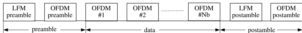
Fig. 8. The structure of the data packet used in the Buzzards Bay experiment, Dec. 15, 2006.
