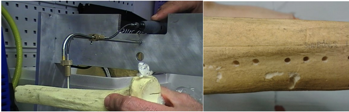
Figure 63: Experimentally testing the performance of the flexible surgical drill system, (left) experiment setup, (right) holes made by the flexible drill.
