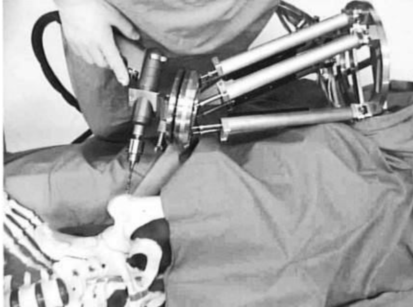
Figure 87: Laboratory setup of the CRIGOS robot to simulate a puncture of a cystic cavity into the femoral head. (Image source: Brandt et al. (121))
