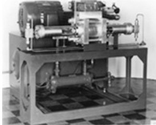
Figure 19: First water jet cutter that installed in Alton Boxboard by N. Franz. (Image source: KMT Water jet)
