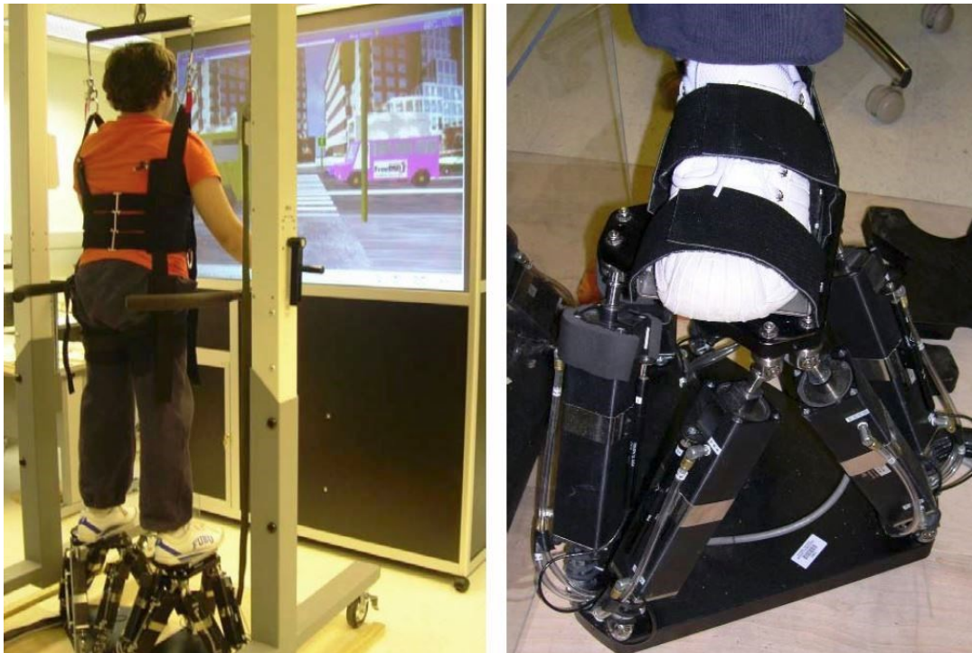
Figure 89: General view of the mobility simulator (left) and The Rutgers Mega-Ankle robot (right). The system simulates walking by moving the platforms back and forth similar to the stepping on a treadmill. (Image source: Boian et al. (124))
