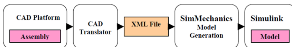
Figure 117: The sequence of CAD to SimMechanics transformation
