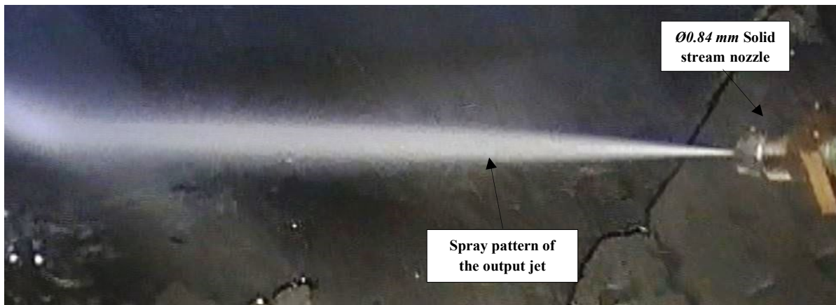
Figure 69: Initial testing of the water jet unit. An excessively-diffuse spray pattern of the output jet was noticed under 10 MPa
