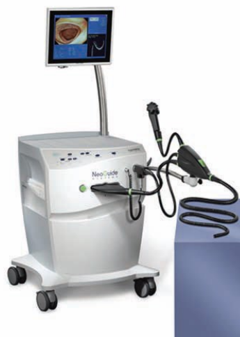
Figure 8: The console of the NeoGuide Endoscopy System contains the video control, light, and insufflation functionality in addition to motors that control the segments in the insertion tube. (Image source: Neoguide Systems Inc. (43))
