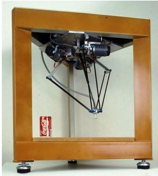
Figure 83: The first ever Delta robot, developed in 1985. (Image source: Clavel (104))
