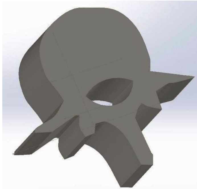
Figure 158: 3-D model of human lumbar vertebrae. The model created in solid works based on image tracing of actual human vertebrae form.
