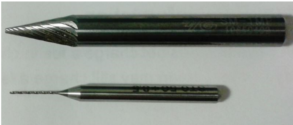
Figure 67: Tools used to fabricate the solid stream nozzle. (Top) carbide burr cone used to machine the conical angle, (bottom) carbide micro-drill bit used to machine the throat of the nozzle.
