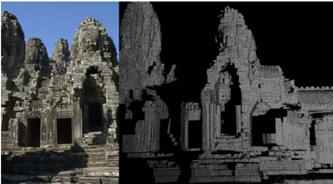
Figure 2.6. A scene for this experiment. Left - a photo of an object; Right - 3D model obtained by the Cyrax-2500 fixed on the ground.
